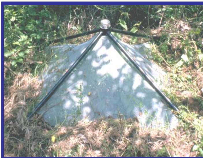
Figure 2. Depiction of a pyramidal emergence trap used for the determination of PC overwintering within two orchard plots in Massachusetts. Trap dimensions: 1.1 x 1.1 yards at base. Traps were purchased from Pest Management Innovations (Harpers Ferry, WV).
