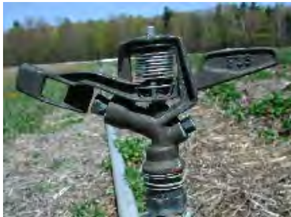
Figure 4: Sprinkler used for frost protection with back nozzle plugged
