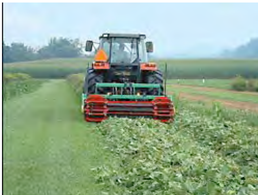
Crimping roller used for elevated beds (for one bed and two furrows) with a customdesigned crimping bar to reach both furrows and a row top. The soybean cover crop (chosen for its ability to fix nitrogen into the soil and form a dense crop canopy) is being rolled and crimped to kill it, forming a mat of dead biomass into which growers can plant a cash crop.
