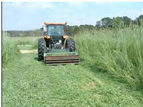
Agricultural engineer Ted Kornecki and his colleagues compared three different roller designs. This roller has a traditional roller with straight horizontal bars.
