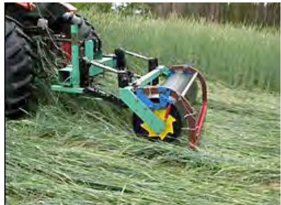
This roller has a smooth drum attached to a crimping bar to smash the rye down as the machine moves forward.
