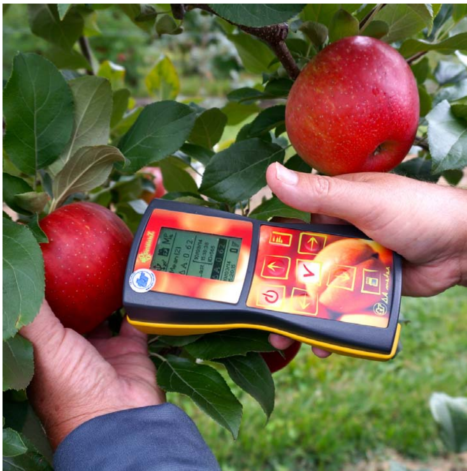
The DA Meter (T.R. Turoni, Italy) measuring 'Honeycrisp' apple maturity at the UMass Cold Spring Orchard, Belchertown, MA. (Photo: Jon Clements, University of Massachusetts)
